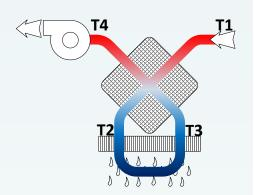
STEP 1 Warm, humid incoming air (T1)flows through the first pass of the plate type air-to-air heat exchangers for pre-cooling and initial dehumidification. This is accomplished by regenerative thermal exchange with the cooler air that is leaving the heat exchanger. (see step 3)
